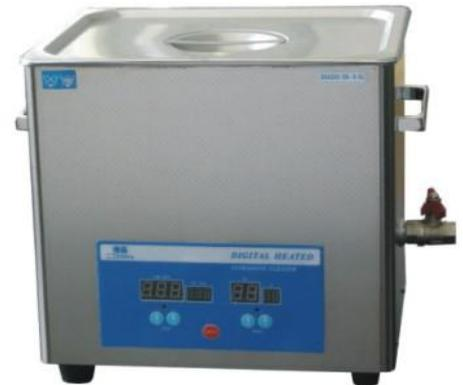
The Ultrasonic energy is produced by converting electrical energy into Mechanical Vibrations by using generator and piezo Electric Transducers. Due to Mechanical Vibrations in cleaning liquid this Phenomenon is called cavitation. In a very short time it removes all dirt & foreign bodies from components which are immersed in the cleaning liquid
